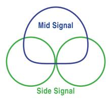
To produce a stereo signal from an M/S configuration, the signal from both microphones must be processed. The PIX recorder can perform this processing on inputs 1 and 2 when Setup Menu option **Audio • Input Linking** is set to **1-2MS**.
