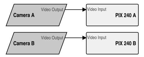
In this scenario, each camera is its own master video sync source, but the PIX is the source of the timecode. The PIX 240i records its files based on the camera's clock. The heads will match perfectly, but the tails may drift depending on the cameras' clocks.
