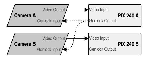
In this scenario, a PIX 240i is the master sync source for multiple cameras, each with or without their own PIX acting as a recorder. Because of this locked connection, the cameras can be run indefinitely and be assured of frame-accurate sync with no possibility of drift.
