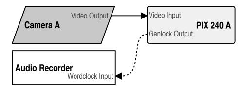
The word clock output on the PIX 240i is synchronous with incoming video signal. The word clock output can be used to sync external audio recorders to any camera. To enable word clock output, set Setup Menu item Timecode/Sync • Sync Out to Wordclock, Follows Video In.
