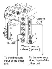
The timecode to be output from the TC OUT connector depends on the setting of "TC Out" on the TC/UB SET menu. If "TC Out" is set to "Generator," the timecode generated by the timecode generator of the camcorder is output during recording and playback. If "TC Out" is set to "Auto," the timecode generated by the timecode generator is output during recording, and that superimposed with the video signal is output during playback.
