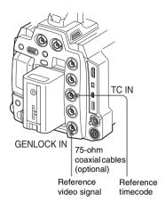
Thus the built-in timecode generator of your camcorder locks to the reference timecode. The message "EXT-LK" is displayed on the screen.
