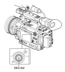
In Slow & Quick Motion mode, the frame rate can be varied by rotating the S&Q dial.
