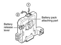
Insert the projection of the battery adaptor into the slot on the rear of the camcorder (0), then lower the ejection lever (0).
